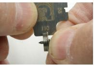
If the measurements N, D, T and W pass, the Inspector now must measure the radii of the fillet between the tread and flange as well as the radii at the outside of the flange. Using a set of radius gauges of the appropriate size and holding the wheel and gauge up to a strong light the Inspector can check that the radius gauge is a good
